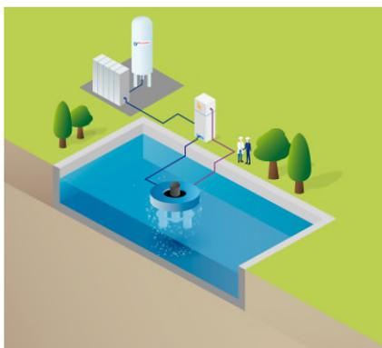
Both systems are installed quickly and easily. They are mobilized with a crane. Power control cabinets and gas cabinets are placed closely to the basins. A monitoring system using a dissolved oxygen sensor can optimize the oxygen quantity which is transferred to the waste water.
