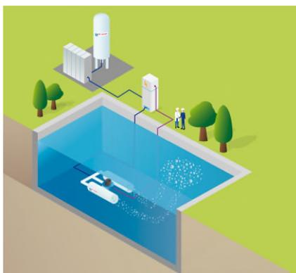
**OXY INJECTOR-TURBOXAL:** floating turbine mixer transfer system designed for treating low bio-degradable pollution and typically shallow basins or lagoons between 2 and 6 meter in depth.
